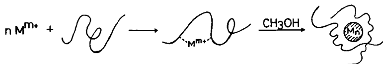
FIG. 1. Schematic presentation of the formation of the colloidal dispersions of noble metal clusters protected by polymers through the polymer-metal complexes.
